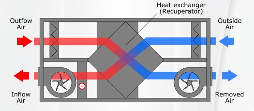
In heating, ventilation and air conditioning systems, HVAC, recuperators are used to reuse released heat from exhaust air, usually expelled to the atmosphere. The heat from the exhaust air flow is transferred into the supply air flow.
